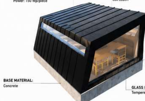
PREFALZ SOLAR MODULE 500 Dimensions: 2,000 x 408 mm Power: 150 Wp/piece
