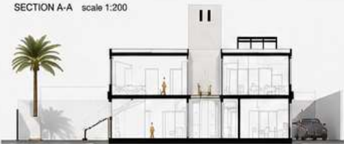
The 12 m high ecological tower expels hot air and draws fresh cool air into the house.
